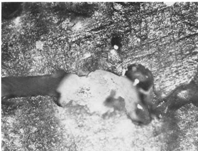
Fig. 4. Void formation after tensile testing around a glass bead coated with a fluorocarbon release agent (magnification 300X).
