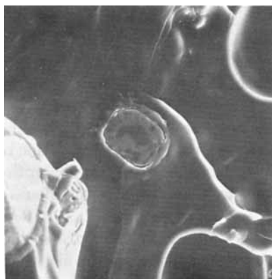
Fig. 14. An ammonium perchlorate particle coated with Silane A-174 in CTPB at the fracture surface (magnification 120\times ).
